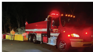
Picture of Engine 1 drafting from 3000-gallon water Tender 1 during a non-hydrant training scenario.
